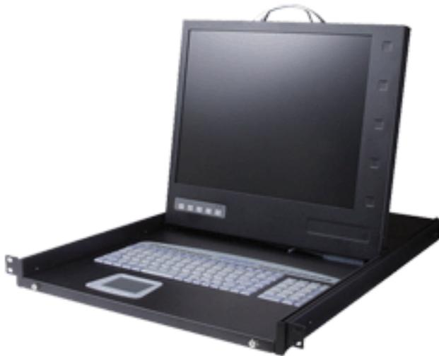
The single-rail modular LCD KVM features an integrated 17"/19"/20" TFT LCD color display, one set of industrial keyboard and touchpad. With the modular design, user only needs to take off few screws and any module can be easily detached/ re-attached again. Module replacement can be implemented with ease. Besides, a 8/16-port KVM module in 1U format design allows user to add to be a 8/16 port LCD KVM in use.
