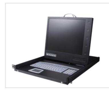
The single-rail modular LCD KVM features an integrated 17" TFT LCD color display, one set of industrial keyboard and touchpad, and a 8/16-port KVM in 1U format. With the modular design, user only needs to take off few screws and any module can be easily detached/ re-attached again. Module replacement can be implemented with ease. Besides, the drawer design allows user to fold and hide the console when not in use.
