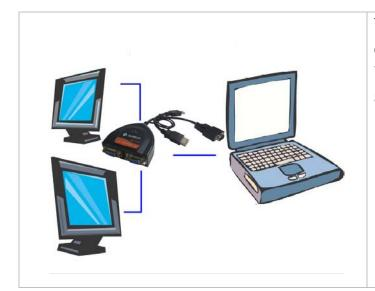
VS-112 Video Duplicator helps boost and duplicate signals from a single source and broadcasts the same signals to 2 monitors from a distance of up to 65meters (210 feet) •
