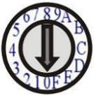
**SE150HX-4K** built in rotary switch for pairing devices and the rotary switch can be used to switch 0-F channel pairing with group setting of switch 1. The channel number and group setting of the transmitter and receiver must be same to be connected each other, total up to 32 (16 for each group) pairs could be setup at one switch.
